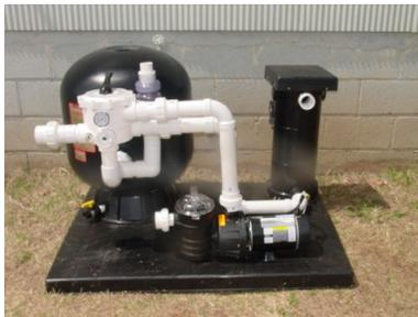
Step 8: Place beads into filter. (See AquaBead manual) Tighten top onto filter using special wrench (included).
