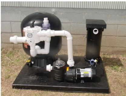
Step 6: Attach pipe from pump to top opening of Multiport valve.
