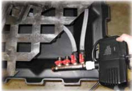
Plug the pump in and adjust valves as needed to desired effect before placing access door in place.
